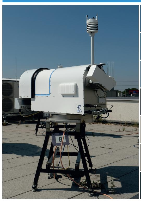
Integrated GPS & automatic weather station
